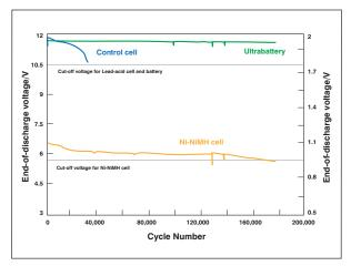
Inserting a supercapacitor into the battery acts as a 'buffer' to manage the high-rate charge/discharge process so that the unit can operate within a state-of-charge window below 70 percent successfully.
